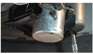
Release and remove the three screws on the pump bracket.
