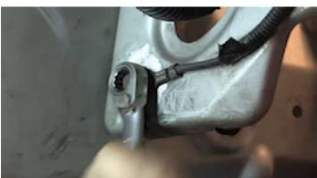
Pull the pump with the bracket from its installation position and disconnect the plug connections. The pump can now by removed from the vehicle.
