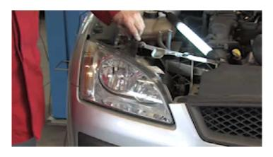
Remove the right headlight according to manufacturer's instructions to gain better access to the pump container.
