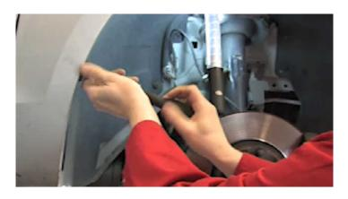
Remove the wheel arch liner at the front right and all panels which could make it more difficult to access the steering pump and its cables.
