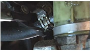
Remove the clamp from the return line using suitable pliers. Pull the return line from the pump.
