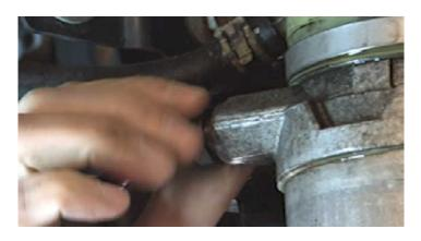
Release the threaded fitting of the pressure line and remove it from the pump.
