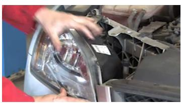
Re-install the headlight, the wheel arch liner and all other removed panels.
