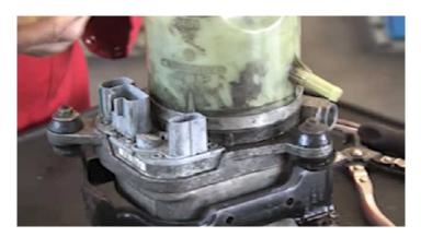
Seal the connections for the hydraulic lines and the connecting socket with the plugs from the supplied replacement pump.
