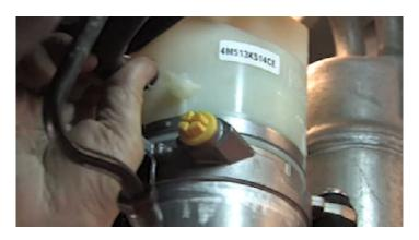
Connect the pressure and return lines to the pump.
