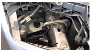
Move the pump with the bracket into the installation position and fix the retaining screws with the torque specified by the vehicle manufacturer.
